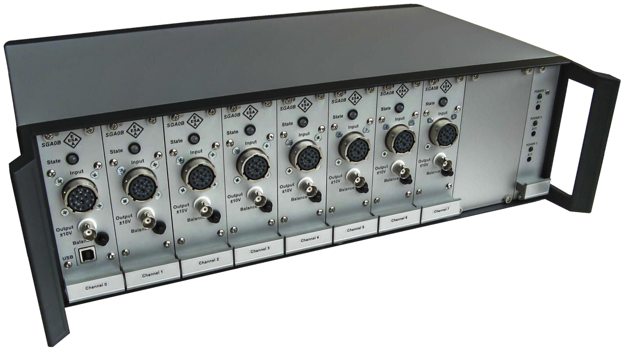
View of an 8-channel amplifier system
