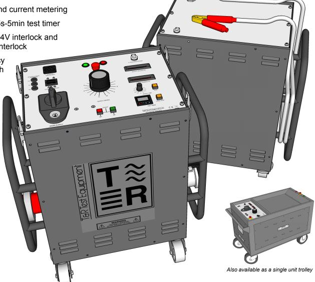
The HV trolley2 series of units are high power AC flash test sets with a 20kVA output capability. The maximum output voltage can be customised to be any voltage up to 15kV. The unit is housed in a rugged aluminium enclosure with a cover to protect the control panel. It is mounted on wheels to allow easy movement within a production environment.
